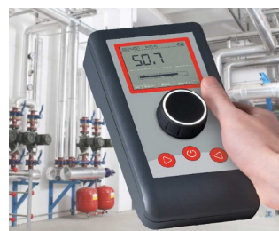
Find compressed air leaks using ultrasound
