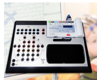
Stationary system for long-term EEG recordings
