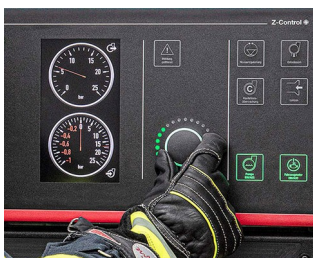
Control element for pump control station
