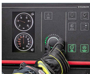
Control element for pump control station
