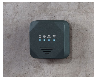
Wireless Access Point
